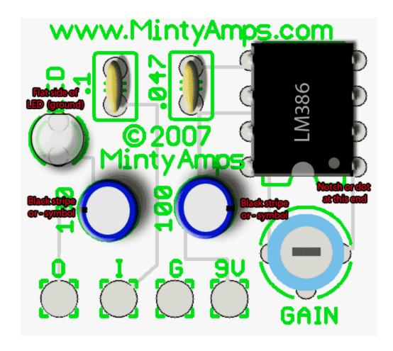
Connect the positive side of the power source to the "9V" pad (via a switch is recommended).
